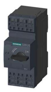
CIRCUIT-BREAKER SZ S0, FOR MOTOR PROTECTION, CLASS 10, A-RELEASE 10...16A, N-RELEASE 208A, SPRING-L. CONNECTION, STANDARD SW. CAPACITY,
