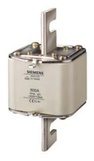
LV HRC FUSE LINK GL/GG WITH NON-INSULATED GRIP LUGS WITH FRONT INDICATOR SIZE 4, 800A, AC 500/DC 440V
