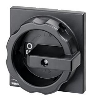
ROTARY ACTUATOR BLACK FOR SWITCH 3LD2, 25A, 32A FOR FRONT MOUNTING FOUR-HOLE MOUNTING
