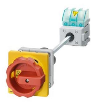
MAIN/EMERG. STOP SWITCH 3-POLE IU=125, P/AC-23A AT 400V=45KW FLOOR MOUNTING DIN RAIL/TWO-HOLE MOUNTING ROTARY ACTUATOR RED/YELLOW (EMERG. STOP)
