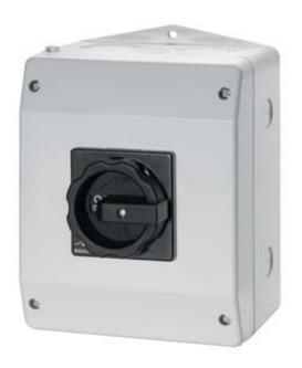
MAIN CONTROL SWITCH 3-POLE IU=100, P/AC-23A AT 400V=37KW 1 N-TERMINAL + 1 PE-TERMINAL ENCAPSUL.IN M.P.ENCLOSURE, IP65 ROTARY ACTUATOR BLACK METRIC THREAD
