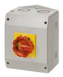
MAIN/EMERG. STOP SWITCH 6-POLE IU=63, P/AC-23A AT 400V=22KW 2 N-TERMINALS INSULATION-ENCLOSED, IP65 ROTARY ACTUATOR RED/YELLOW (EMERG. STOP)
