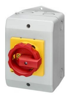
EMERG. STOP SWITCH 3-POLE IU=63, P/AC-23A AT 400V=22KW 1NO+1NC, 1 N-TERMINAL INSULATION-ENCLOSED, IP65 ROTARY ACTUATOR RED/YELLOW (EMERG. STOP) METRIC SCREW CONNECTION
