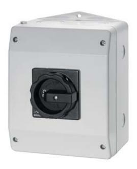
MAIN CONTROL SWITCH 3-POLE IU=63, P/AC-23A AT 400V=22KW 1NO+1 NC, 1 N-TERMINAL ENCAPSUL.IN M.P.ENCLOSURE, IP65 ROTARY ACTUATOR BLACK METRIC THREAD
