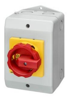
EMERG. STOP SWITCH 3-POLE IU=63, P/AC-23A AT 400V=22KW 1 N-TERMINAL + 1 PE-TERMINAL INSULATION-ENCLOSED, IP65 ROTARY ACTUATOR RED/YELLOW (EMERG. STOP) METRIC SCREW CONNECTION
