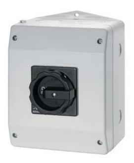
MAIN CONTROL SWITCH 3-POLE IU=63, P/AC-23A AT 400V=22KW 1 N-TERMINAL + 1 PE-TERMINAL ENCAPSUL.IN M.P.ENCLOSURE, IP65 ROTARY ACTUATOR BLACK METRIC THREAD
