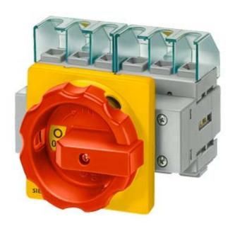
EMERG. STOP SWITCH 6-POLE IU=63, P/AC-23A AT 400V=22KW FRONT MOUNTING FOUR-HOLE MOUNTING ROTARY ACTUATOR RED/YELLOW (EMERG. STOP)
