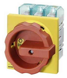
EMERG. STOP SWITCH 3-POLE IU=63, P/AC-23A AT 400V=22KW FRONT MOUNTING FOUR-HOLE MOUNTING ROTARY ACTUATOR RED/YELLOW (EMERG. STOP)
