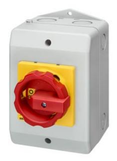
EMERG. STOP SWITCH 4-POLE IU=32, P/AC-23A AT 400V=11.5KW 1 N-TERMINAL INSULATION-ENCLOSED, IP65 ROTARY ACTUATOR RED/YELLOW (EMERG. STOP) METRIC SCREW CONNECTION
