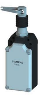
SIRIUS CABLE-OPERATED SWITCH METAL ENCLOSURE; 2XM20X1.5 1NO+1NC, WITHOUT LATCH CABLE-OPERATED FUNCTION ONLY MAX. ACTUATING FORCE 80N ACTUATING FORCE 80N MAX.
