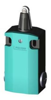
SIRIUS POSITION SWITCH 3SE5162, METAL HOUSING XL, WIDTH 56MM ROLLER PLUNGER, WITH HIGH-GRADE STEEL ROLLER 13MM DEVICE CONNECTION 3X(M20X1.5), 2X (1NO/1NC ) SNAP ACTION CONTACTS IP66/IP67 IP66/IP67
