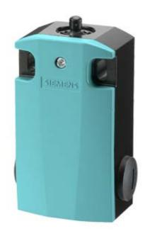
BASIC SWITCH FOR POSITION SWITCH 3SE5162, METAL ENCLOSURE XL,56MM WIDE DEVICE CONNECTION 3X(M20X1.5), IP66/IP67 2X (1NO/1NC) QUICK ACTION CONTACTS, WITHOUT ACTUATOR HEAD
