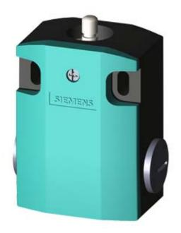
BASIC SWITCH FOR POSITION SWITCH 3SE51, METAL ENCLOSURE 56MM, TO EN50041 3X(M20X1.5) 1NO/ 2NC SLOW-ACTION CONTACTS W/O ACTUATOR HEAD
