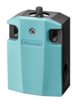
BASIC SWITCH W. INCREASED CORROSION PROTECTION FOR POSITION SWITCH 3SE51, METAL ENCLOSURE 56MM, DEVICE CONNECTION 3X(M20X1.5), 1NO/ 1NC SNAP-ACTION CONTACTS W/O ACTUATOR HEAD
