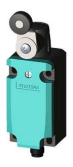
TO EN50041 1NO/ 1NC SNAP-ACTION CONTACTS W. M12 CONNECTOR, 5-POLE, FIXED PIN ASSIGNMENT: PIN1=21, PIN2=22, PIN3=13, PIN4=14, PIN5=PE ROTARY ACTUATOR RIGHT AND/ OR LEFT ADJUSTABLE, METAL LEVER 27 MM LONG AND PLASTIC ROLLER
