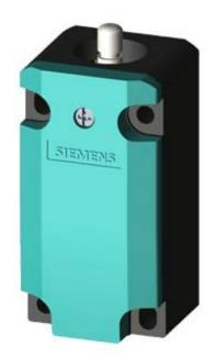
BASIC SWITCH FOR POSITION SWITCH 3SE5112, METAL ENCLOSURE, TO EN50041, 40 MM; 1X(M20X1.5) 1NO/2NC SLOW-ACTION CONTACTS WITH OVERLAP W/O ACTUATOR HEAD
