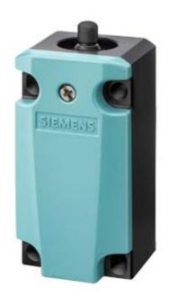
BASIC SWITCH FOR POSITION SWITCH 3SE51, METAL ENCLOSURE, ACC. TO EN50041 DEVICE CONNECTION 1X (M20X1.5) 1NO/2NC SNAP-ACTION CONTACTS W/O ACTUATOR HEAD
