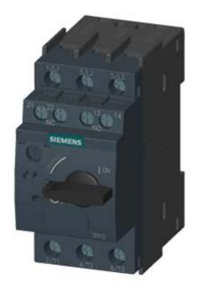
CIRCUIT-BREAKER SZ S00, FOR MOTOR PROTECTION, CLASS 10, A-RELEASE 9..12.5A, N-RELEASE 163A, SCREW CONNECTION, STANDARD SW. CAPACITY W. TRANSVERSE AUX. SWITCH 1NO+1NC
