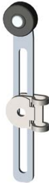
LENGTH-ADJUSTABLE TWIST LEVER FOR POSITION SWITCH 3SE51/52 METAL LEVER 100MM LONG PLASTIC ROLLER 19MM
