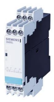
COUPLING RELAY IM INDUSTRY-STANDARD ENCLOSURE 2 CHANGEOVER CONTACTS COMBIVOLTAGE 24 V AND 220 V TO 240 V AC/DC SCREW TERMINALS
