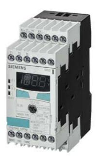
TEMPERATURE MONITORING RELAY PT100/1000, KTY83/84, NTC 3 SENSORS, 2 THR. VAL., DIGITAL -50 DEG. C TO 500 DEG. C 24-240V AC/DC 2 X 1 W + 1 NO, WIDTH 45 MM SCREW CONNECTION
