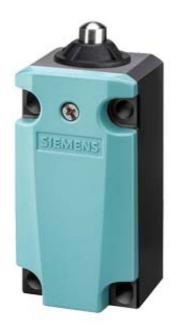
SIRIUS POSITION SWITCH, METAL ENCLOSURE 40MM, TO EN50041 DEVICE CONNECTION 1X (M20X1.5) 1NO/1NC SLOW-ACTION CONTACTS PLAIN PLUNGER, STAINLESS STEEL
