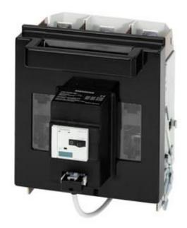
FUSE-SWITCH-DISCONNECTOR I=400A, U=690V, AUXILIARY SWITCH 1NO+1NC FOR CABLE-LUG CONNECTION FUSE SIZE NH1 AND NH2 WITH FUSE MONITORING BY 3RV, WITH 1NO+1NC
