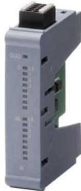
SIMATIC S7-1200 G2: SB 1233 analog I/O, 2 AI/2 AO inputs: 2 x AI 14 bit ADC (+/-10 V, +/-5 V, +/-2.5 V or 0-20 mA/4-20 mA) outputs: 2 x AQ 14 bit DAC (+/-10 V, 0-20 mA or 4-20 mA)
