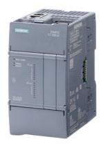
SIMATIC S7-1200 G2: compact CPU 1212C AC/DC/RLY; power supply: AC 85-264 V AC at 47-63 Hz; onboard I/O: 8x DI 24 V DC; 6 DO relay 2 A; memory: program 150 KB data: 500 KB, retentivity: 20 KB
