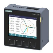
SENTRON PAC4220, Power Monitoring Device with color graphic TFT display PMD-III acc. to IEC61557-12 active energy class 0.2 (class 0.2S acc. to IEC62053-22) 96 x 96 mm, 3-phase, 45 - 65 Hz Ue rated: 690/400 V Ie rated: x/1A or x/5A DC extra-low voltage power supply unit 24 to 48 V +-25% screw terminal connection control panel instrument with measurement of electrical variables apparent / active / reactive energy / cos phi / THDu / THDi / even and odd harmonics per phase up to 64.
