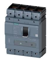
circuit breaker 3VA1 IEC Frame 400 breaking capacity class S Icu=36 kA @ 415 V 4-pole, line protection TM240, ATAM, In=400 A overload protection Ir=280 A...400 A short-circuit protection Ii=5...10 x In neutral conductor protection 100% nut keeper kit
