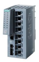
SCALANCE XC208EEC manageable Layer 2 IE switch; IEC 62443-4-2 certified; 8x 10/100 Mbit/s RJ45 ports; 1x console port; diagnostics LED; redundant power supply; with painted printed-circuit boards; NAMUR NE21-compliant; temperature range -40 °C to +70 °C; assembly: DIN rail/S7 mounting rail/wall; redundancy functions; Office; features (RSTP, VLAN,...); PROFINET IO device; Ethernet/IP-compliant; C-PLUG slot;
