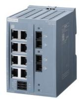
SCALANCE XB108-2 unmanaged IE switch, 8x 10/100 Mbit/s Ports, 2x 100 Mbit/s multimode SC, for setting up small star and line topologies; LED diagnostics,IP20, redundant power supply, 24 V AC/DC Manual available as a download .
