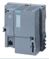
SIMATIC DP, CPU 1514SP F-2 PN for ET 200SP, central processing unit with work memory 900 KB for program and 3.5 MB for data, 1st interface: PROFINET IRT with 2-port switch, 2nd interface: PROFINET RT, 6 ns bit performance, SIMATIC Memory Card required, BusAdapter required for 1st interface \*\*\*\* approvals and certificates according to ID 109818872 at support.industry.siemens.com to be observed! \*\*\*\*
