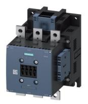
power contactor, AC-3e/AC-3 265 A, 132 kW / 400 V AC (50-60 Hz) / DC Uc: 220-240 V 3-pole, auxiliary contacts 2 NO + 2 NC drive: conventional main circuit: busbar control and auxiliary circuit: spring-loaded terminal
