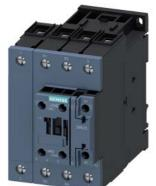
Power contactor, AC-3 40 A, 18.5 kW / 400 V 2 NO + 2 NC 24 V AC, 50 Hz 4-pole size S2 screw terminals 1 NO + 1 NC integrated
