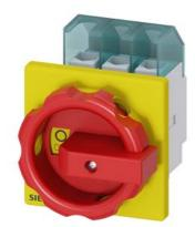
SENTRON, Switch disconnector 3LD, emergency switching-off switch, 3-pole, Iu: 25 A, operating power / at AC-23 A 400 V: 9.5 kW, front-mounted, rotary operating mechanism, Red / yellow, 4-hole mounting of the handle
