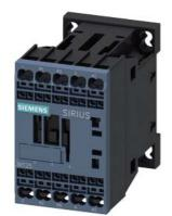
Contactor, 2NO + 2NC, AC-3, 5.5 kW, 110 V AC, 50 / 60 Hz, 4-pole, 2NO + 2NC, Size S00, Spring-type terminal Full-wave rectifier integrated
