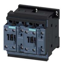
Reversing contactor assembly AC-3,18 kW/400 V,AC230V,50/60Hz 3-pole, Size S0 screw terminal electrical and mechanical Interlock 2 NO integrated
