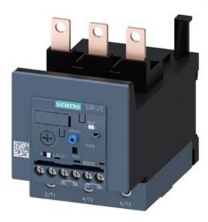
Overload relay 32...115 A Electronic For motor protection Size S3, Class 10E Contactor mounting Main circuit: Screw Auxiliary circuit: Screw Manual-Automatic-Reset
