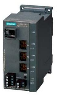
SCALANCE X201-3PIRT managed IE IRT switch, 1x 10/100 Mbit/s RJ45 ports, 3x 100 Mbit/s POF SC RJ ports, Error signaling contact with set button, Redundant power supply, PROFINET IO device, network management, Redundancy Manager integrated, incl. electron. manual on CD-ROM, C-plug optional
