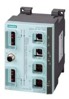
SCALANCE X202-2PIRT PRO, Managed IE IRT switch, Degree of protection IP65/67, 2x 10/100 Mbit/s Push Pull RJ45 ports, 2x 100 Mbit/s Push-pull SCRJ port; Error signaling contact with set button, Redundant power supply, PROFINET IO device; network management, Redundancy Manager integrated, incl. electron. manual on CD-ROM, C-plug optional
