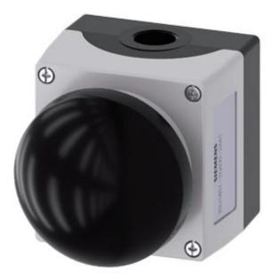
Enclosure for command devices 22 mm, round, Enclosure material metal, enclosure top part gray, 1 control point metal, Control point in center, A = palm pushbutton, black, momentary contact type, 1 NO, screw terminal, Floor mounting
