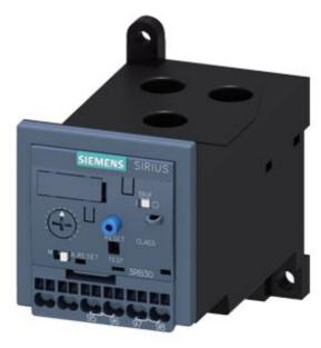
Overload relay 12.5...50 A Electronic For motor protection Size S2, Class 10E Stand-alone installation Main circuit: Straight-through transformer Auxiliary circuit: Spring-type terminal Manual-Automatic-Reset
