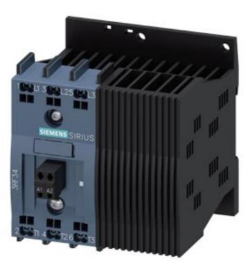
Solid-state contactor 3-phase 3RF3 AC 53 / 12.5 A / 40 °C 48-480 V / 24 V DC 2-phase controlled Instantaneous switching Spring-type terminal
