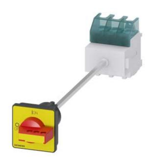
SENTRON, switch disconnector 3LD, EMERGENCY OFF switch, 3-pole, lu: 63 A, Operating power / at AC-23 A at 400 V: 22 kW, floor mounting with door coupling, defeatable knob-operated mechanism, red/yellow, 4-hole mounting of the handle
