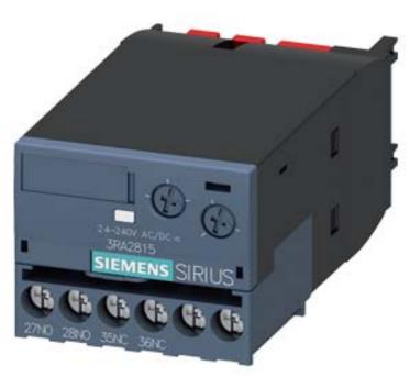
Solid-state time-delayed auxiliary switch OFF delay without control signal Relay 1 NC + 1 NO 24...240 V AC/DC Time range 0.05...100 s can be snapped on at the front for contactors 3RT2 S00-S3 Screw terminal Varistor for attenuation of the contactor coil integrated
