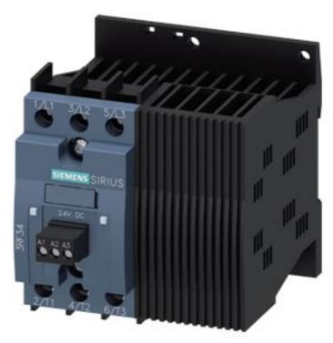
Solid-state contactor 3-phase 3RF3 AC 53 / 7.4 A / 40 °C 48-480 V / 24 V DC Reversing circuit Instantaneous switching screw terminal
