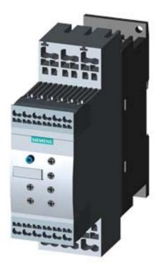
SIRIUS soft starter S0 38 A, 18.5 kW/400 V, 40  $^{\circ}$ C 200-480 V AC, 24 V AC/DC spring-type terminals Thermistor motor protection
