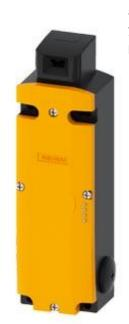
Safety position switch with tumbler Locking force 2600 N 5 directions of approaches Solenoid-locked Magnet voltage 115 V AC Monitoring actuator 2 NC/1 NO Monitoring magnet 2 NC/1 NO LED display yellow/green Supplied without actuator. Actuator 3SE5000-0AV0. please order separately
